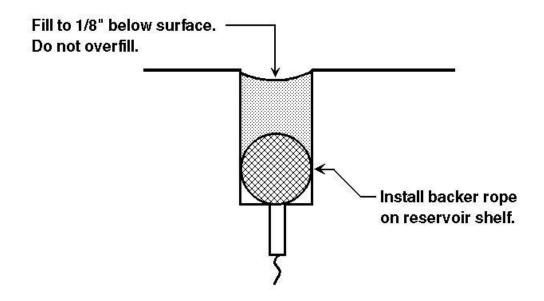
Figure 6. PCC joint/crack repair.
