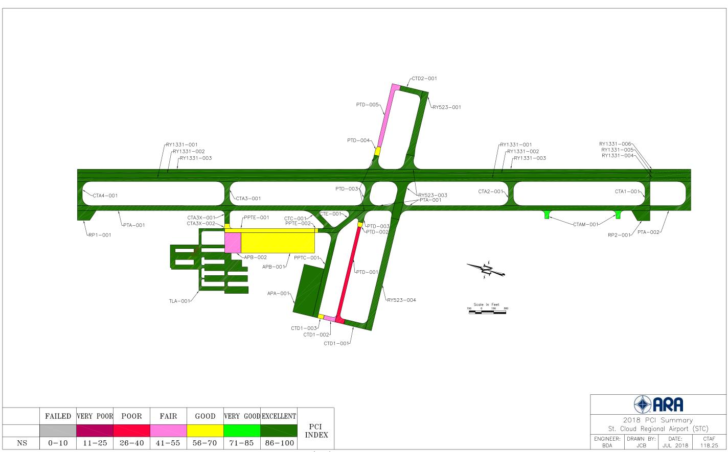
Figure 4. 2018 Pavement Condition Index Rating at St. Cloud Regional Airport (STC).
