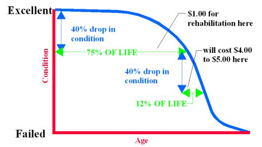
Figure 1. Pavement condition life cycle.
