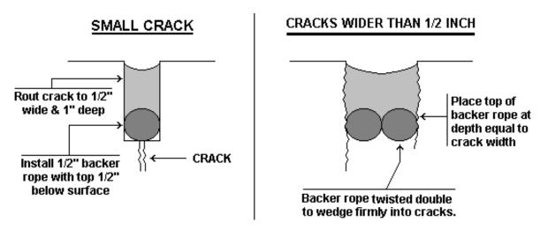
Figure 2. Crack sealing.
